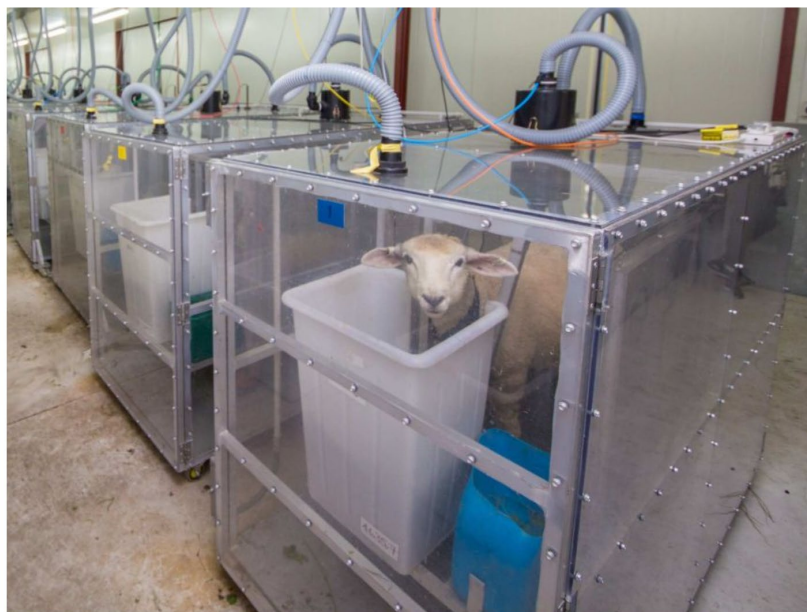
Figure 7: Emissions accumulation chamber with sheep (Daly, 2018)
